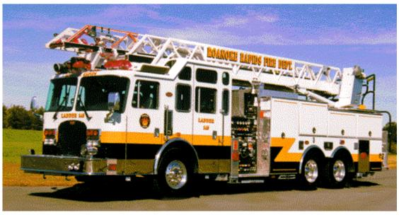
The Roanoke Rapids Fire Department's newest piece of equipment – Ladder #145 – was delivered in November 1998. It is a 75-foot, three-section AerialCat powered by a 500-horse power Cummins diesel engine with an Allison Transmission custom built to the City's specification. It is equipped with a 1,500 gallons per minute single stage pump, a 500-gallon poly water tank and 30-gallon foam tank.
